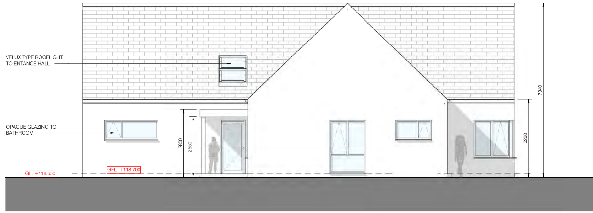
2 House Type 01 - North Elevation 1 : 100
