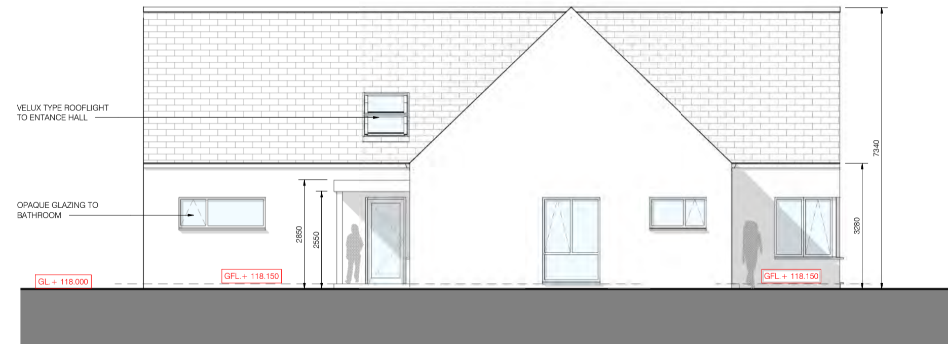
5 House Type 02 - West Elevation 1 : 100
